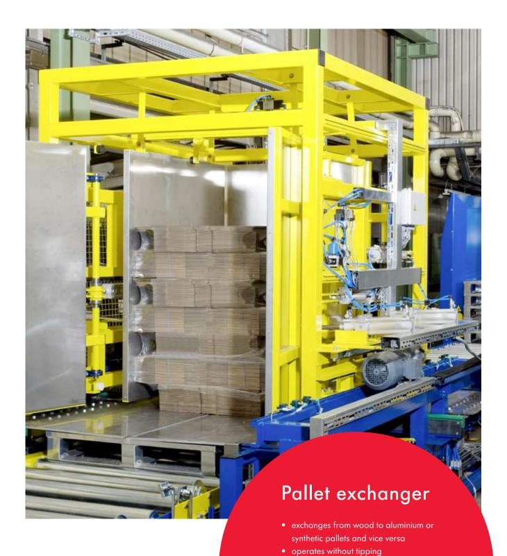
exchanges even fragmentary loadsup to 60 exchanges per hour
